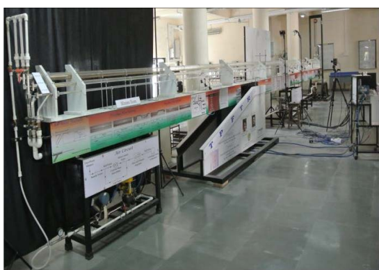
LDV Analysis of Air-Water Two-Phase Flow In Horizontal Pipe
