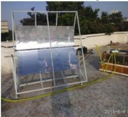
Solar Thermal- Parabolic Trough with Active tracking
