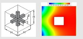
In order to estimate the volumetric heat transfer coefficient and thermal dispersion coefficient of the representative foam structure, pore level simulations were carried out in the commercial solver ANSYS-Fluent. The required mesh files were generated in ICEM tool. The employed numerical models are further utilized to determine the functional dependency of Nusslet number and dispersion coefficient on Reynolds number, Prandtl number, and porosity. **Project B**
